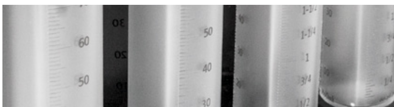
EACH TUBE'S CAPACITY IS 90 ML OR 3 OZ, IN INCREMENTS OF 1 ML / 0.3 OZ
